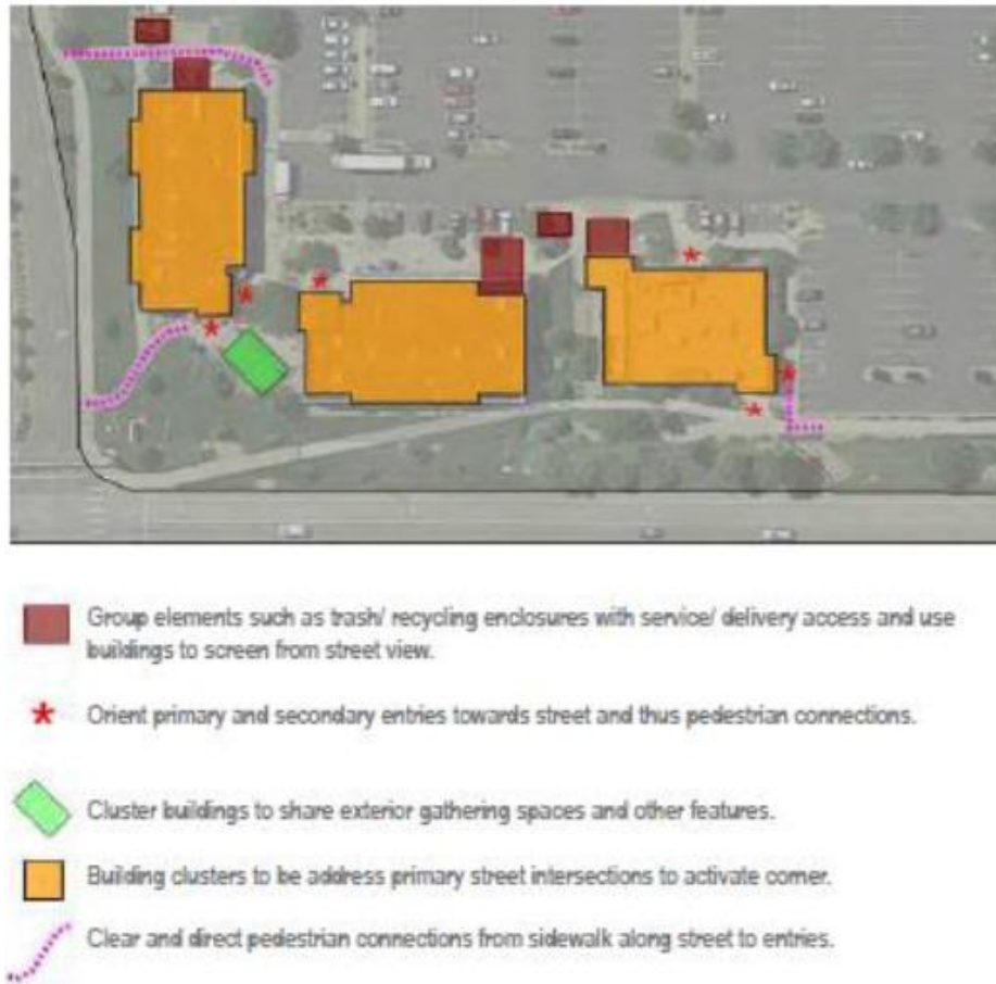
Figure 3.9: Building Placement Example
